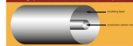
Pic.4 Dupont® Nomex® IIIA fabric includes P-140 - a kind of high-performance static-eliminated fiber with patent.
